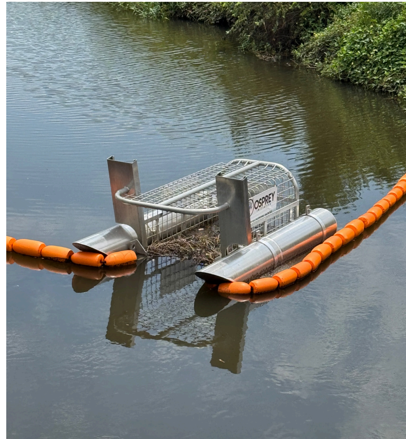
Litter Gitter Installation
