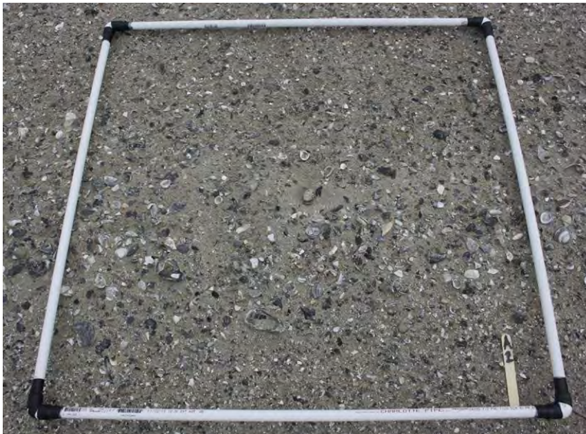
Figure 4. Placement of PVC grid and nest marker used to document the unique nest code and physical nest habitat characteristics.
