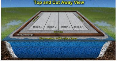
**Stormwater Infiltration Basin and Petanque Terrain**
