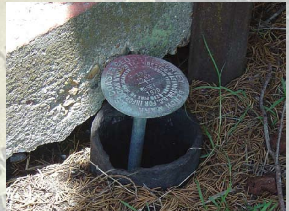
Subsidence leaves a south Louisiana benchmark standing above current ground level.
